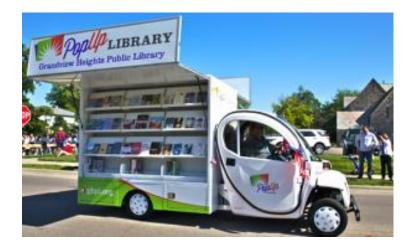
This mobile library is a low-speed, electric vehicle that can travel up to 25-30 miles on a single charge, with a maximum speed of 30 mph. It is especially customized to transport
